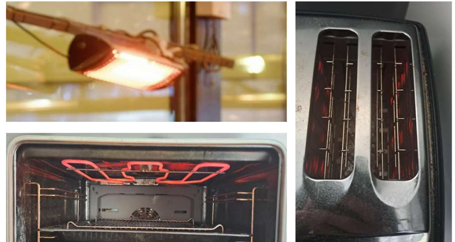
heating elements in an IR heater, toaster and grill
